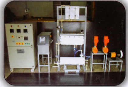
Electro Chlorination Plant
