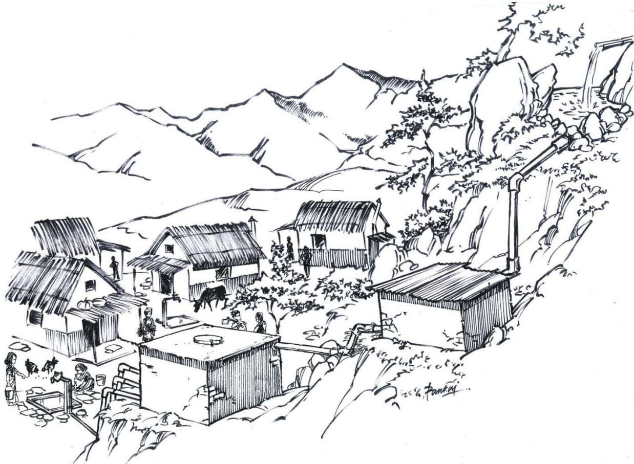
Figure 3: Typical Gravity Fed Piped System
